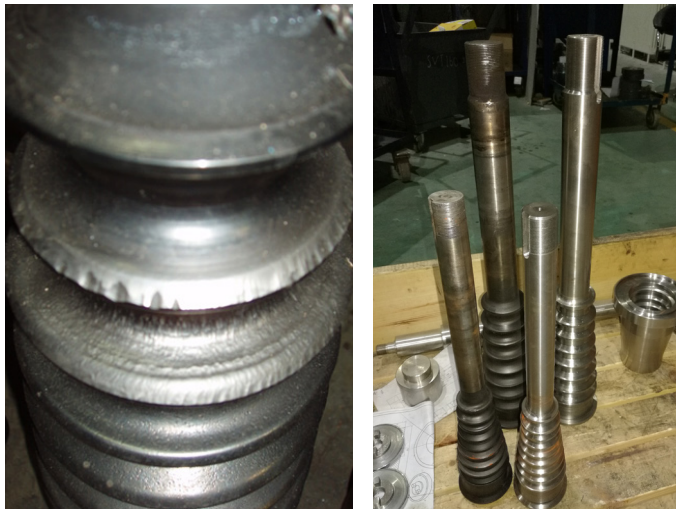
Damaged multistage valve trim with new replacement trim engineered and manufactured by WZI.
